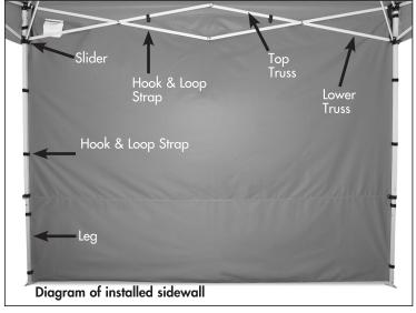
**Step 2.** Attach sidewall to frame as shown. (2a) Wrap hook and loop straps around the top truss.
