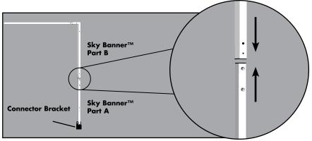
**Step 7.** Attach the Connector Brackets onto both shelter frame legs approximately 16" below the already installed fixed connector bracket.
